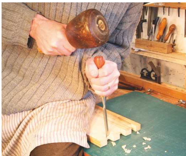
▲ Pic.11 Cleaning up to the line: a very slight undercut will help
